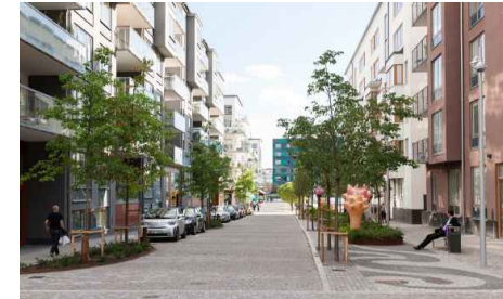
Figure 147: Narrow local streets - flush pavements - enhanced pedestrian/cycle priority. Source: https://cmgrannis.medium.com/hammarby-sj%C3%B6stad-stockholm-sweden-894e6cc2dcfa
