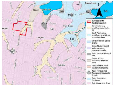
Figure 5: The geology is Ashfield Shale and soils are of the Blacktown Soils Landscape. Quaternary-period valley infills mark the alignment of the unnamed Aboriginal watercourse that originally crossed the land. Source: Burwood North Masterplan First Nations Design Precincts Report
