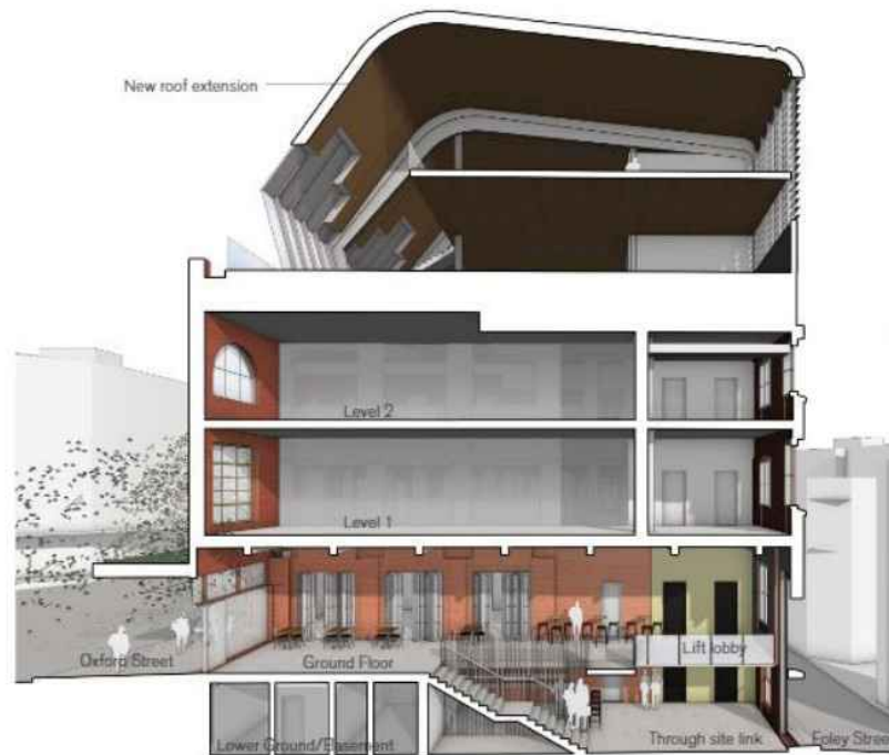
Figure 108: Adaptive re-use - mixed-use maintaining high street character - activation of rear laneway. Source: FJMT Architects
