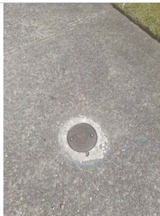
Photo 8: Monitoring well visible on the pavement of Parramatta Road adjacent to the 7-Eleven Petrol Station.
