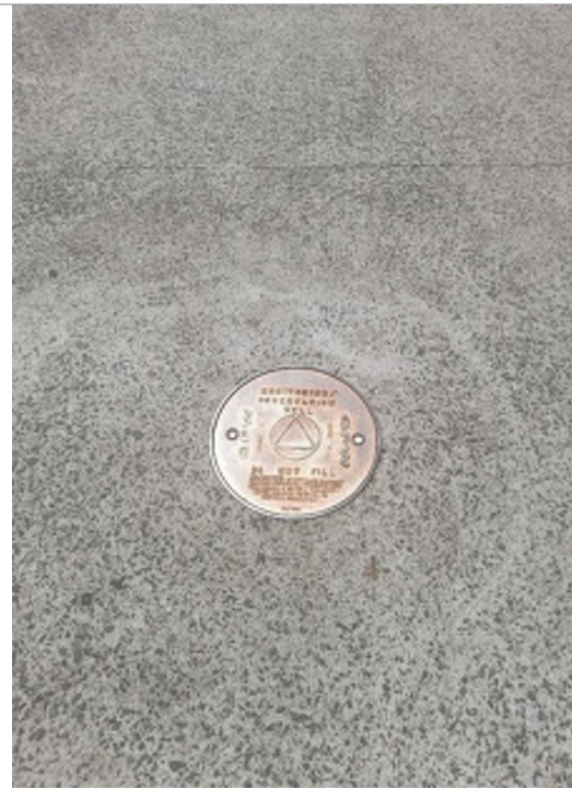
Photo 14: Monitoring well located within Ampol Petrol Station (east of the station adjacent to Park Road).
