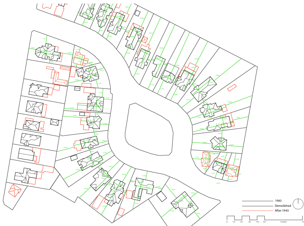
Figure 8 – Diagram showing original (or early) building footprints) with alterations since 1943. Demonstrating the highly intact group of dwellings. Jennifer Hill.
