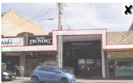
Drastic changes in height that break the continuity of the awning alignment with the rest of the streetscape are discouraged.
