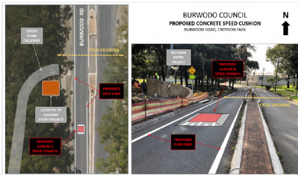
PROPOSED CONCRETE SPEED CUSHION
