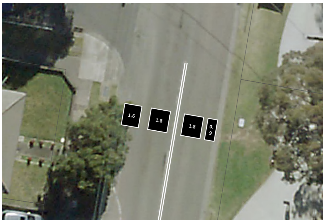
Portland Street Rubber Speed Cushion Placement
